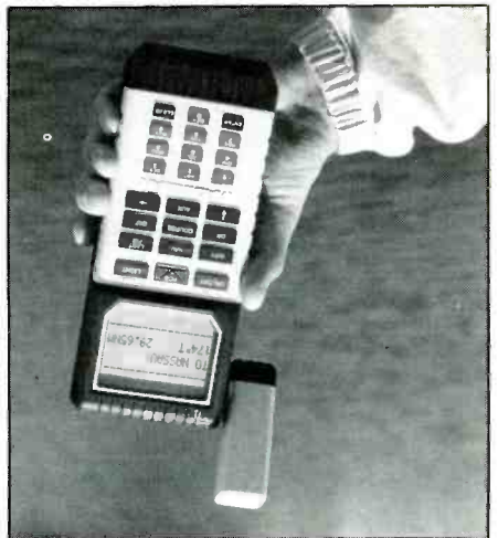
The portable Magellan receiver will also indicate direction to a stored "Way Point." Courtesy Gordon West.
