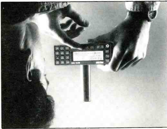
Portable GPS receiver reads out position and bearings within 300 yard accuracy. Note small 1.5 GHz antenna on top of portable GPS set. Courtesy Gordon West.
